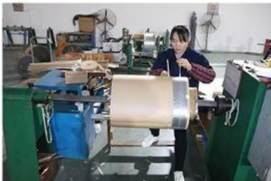
HV Coil Winding
